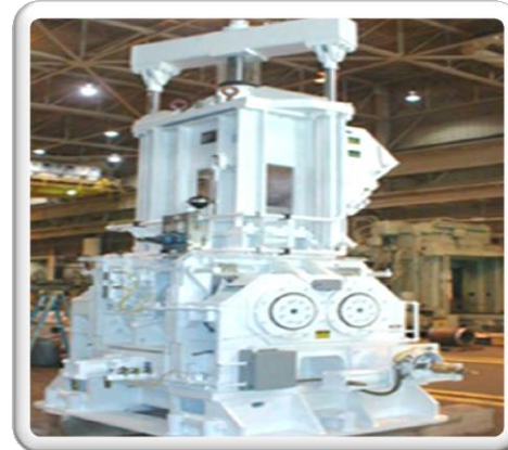
Banbury mixer/ Kneading action/melting Farrel (5 to 10 min)
