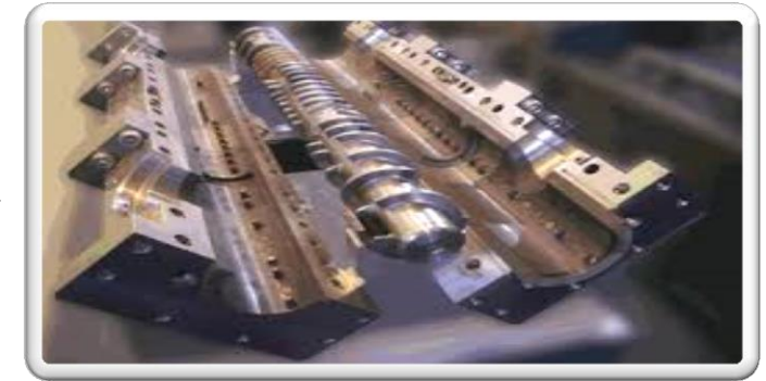
Co – Kneader/stirring action Buss and B&P Systems (5-8min)
