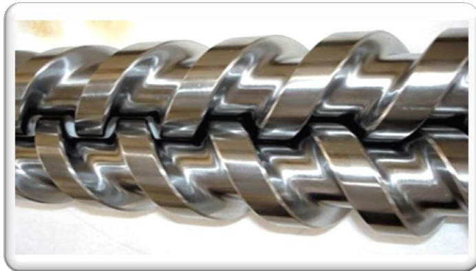
Counter rotating twin extruder/ Elongational mixing 1907-1955
