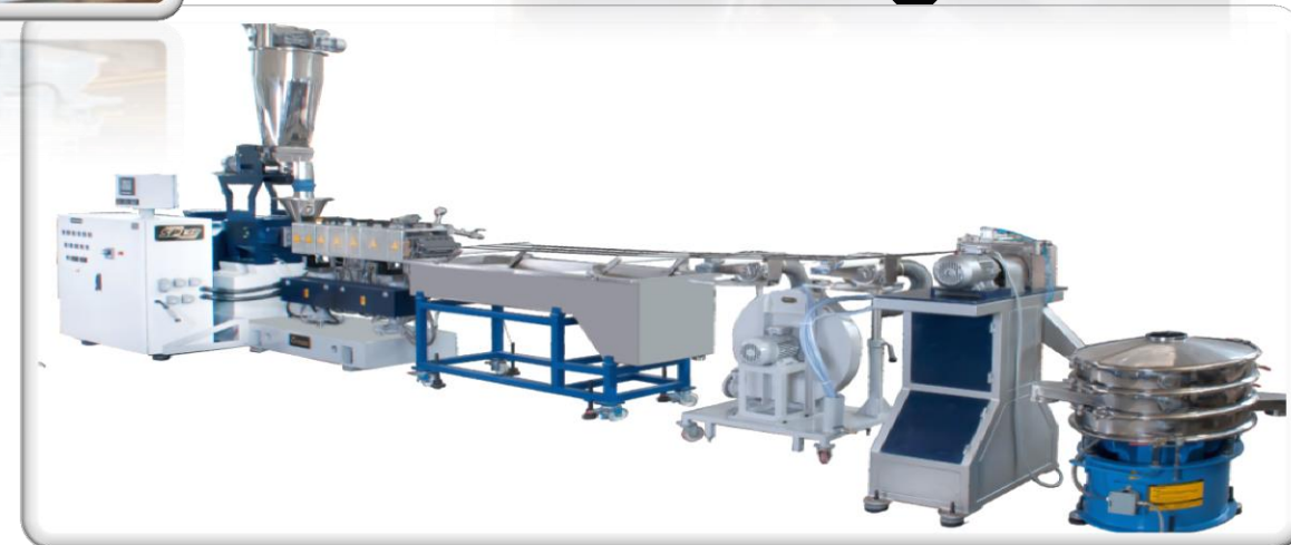
Twin screw extruder residence time 3-4 min
